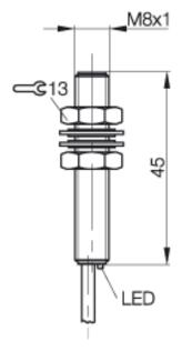
Inductive Sensors BES 516-377-EO-C-02 M8x1 x 46.5 normally-closed Sn=1,5mm shielded
